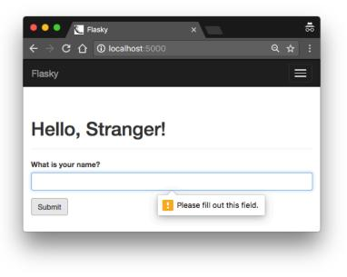
Figure 4-3. Web form after failed validator
